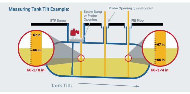
Stick the tank at the **Probe Opening in the STP Sump**, at the **Fill Pipe**, and at the separate **Probe Opening** (*if applicable*) to determine tank tilt. Place the stick heights on the tank diagram below next to each location to the nearest eighth of an inch. Please be as precise as possible. An additional measurement from the bottom of the tank to the top of the **Manway Fitting** will also be needed. (This dimension may be obtained from the tank drawing if detail is available.)
