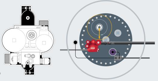
**Observe the Fuel Conditioner measurements in the example below.** Take a top down picture of the sump using the "True to Size" Fit Test Model in place over the intended bung.
