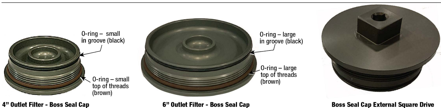
Figure 4. O-Ring Locations for Boss Seal Cap w/External Square Drive
